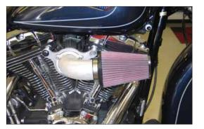
13. Install the K&N air filter onto the intake tube and secure with the provided hose clamp.
