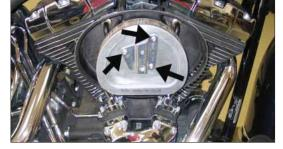
3. Remove the three air filter retaining bolts shown.
