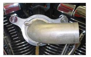
12. Install the K&N intake tube with the gasket and secure with the provided hardware. **NOTE: Apply one drop of the provided thread locker onto the provided bolts.**
