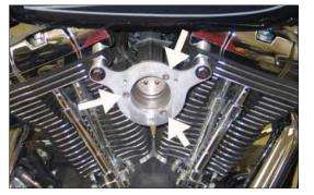
11. Install the provided gasket between the throttle body and back plate and then secure the back plate to the throttle body with the hardware provided. Tighten the crank case breather bolts. **NOTE: Apply one drop of the provided thread locker onto the provided bolts.**
