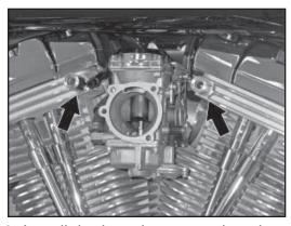
13. Install the breather extensions into the stock breather bolt location as shown.
