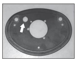
7. On vehicles equipped with a carbon canister, drill a 5/8"ID hole in the backing plate at the marked location from the previous step.
