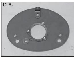
11. Install the three stand-offs onto the backing plate using the three bolts from the previous step.
