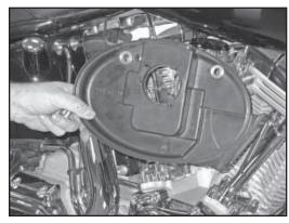
4. Remove the stock air filter base from the engine as shown.
