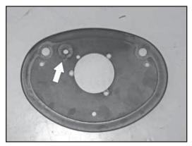
8. On vehicles equipped with a carbon canister, install the provided grommet into the backing plate as shown.
