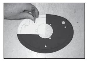
6. Some vehicles are equipped with a carbon canister vent line that connects into the backing plate. Use the provided template to mark the K&N backing plate drilling location as shown.
