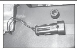
5. Some models are equipped with an intake valve solenoid connector on the back of the stock air filter back plate. Unhook the connector from back plate.
