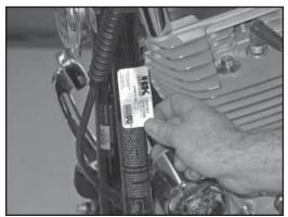
21. Install the E.O. sticker near the vehicle emissions label as shown.
