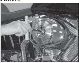
1. Remove the air filter cover mounting bolt and cover from the vehicle as shown.
