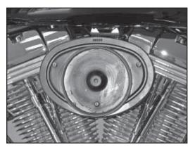
19. Install the K&N air filter and secure with the three bolts provided.
