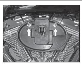
3. Remove the stock breather bolts which secure the stock air filter base shown.
