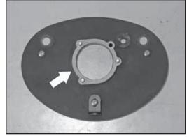
14. Install the provided gasket onto the K&N backing plate as shown.
