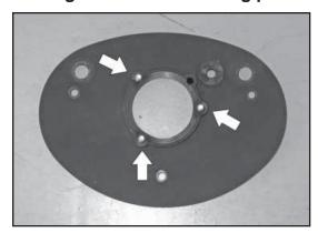
10. Install the three backing plate mounting bolts through the velocity stack as shown.
