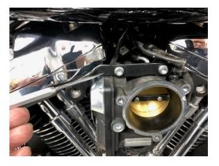
1B) Remove factory throttle body support bracket
