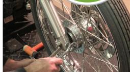
3. First loosen the axle nut, and then the pinch bolt in the bottom of the right fork lower leg, and remove the front wheel.
