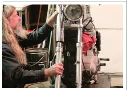
7. Slide tube back into the trees and check installed height of tubes at the top tree. Torque pinch bolts to factory specifications.
