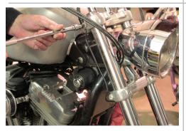
4. Loosen the top and bottom pinch bolts on the triple trees (one side at a time) and remove the bolts- be sure to hold the fork tube as it will fall out if not supported.
