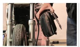
Remove the front fender. IMPORTANT NOTE: the fender cannot be used with the fork covers.
