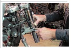
6. Install fork cover. The spacers will go on the bottom; in-between the tab on the shroud and the bottom triple tree.
