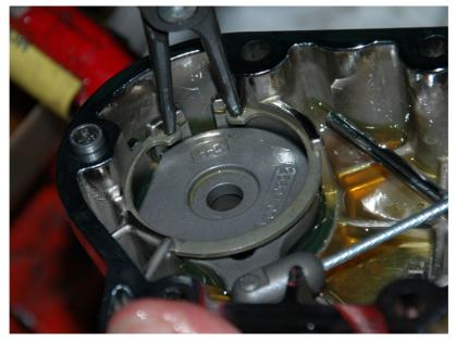
Remember the exact position of the retaining clip before you start to remove this clip (later it has to be fitted at the same position to the gap in the cover).
