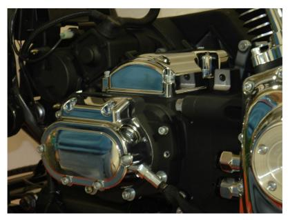
Check the transmission case cover on the right side of your bike and remove your exhaust system in case it is covering the transmission cover.
