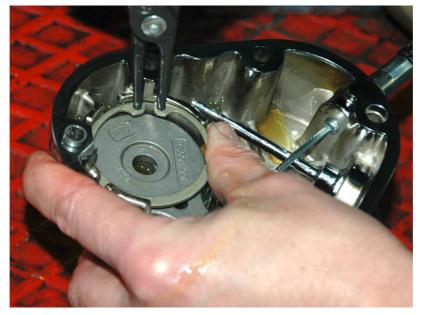
Insert the retaining ring now but watch your fingers! After that, turn the retaining ring until it has reached the original position.
