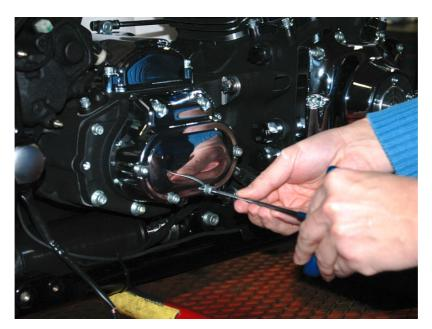
Take a clean oil bowl and put it below the transmission cover and then start removing the six screws of the transmission cover carefully with a x/x allen wrench.
