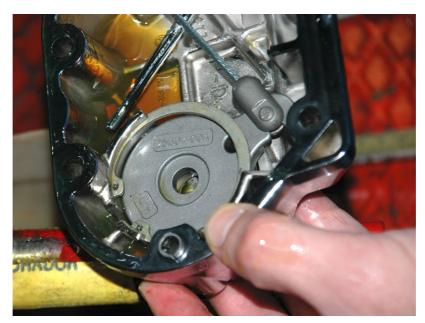
Look at the inside of the removed cover and see the OEMclutch drive unit. The inner plate will be exchanged with the Clutchlite.
