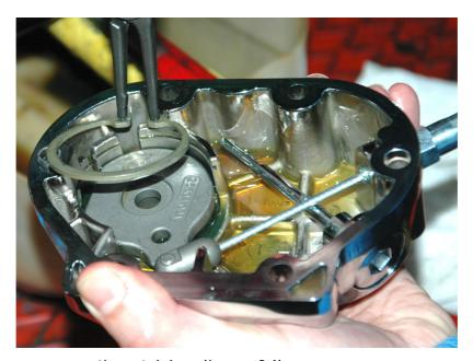
... remove the retaining clip carefully.
