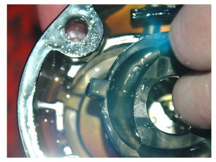
Take both clutch drive plates out and exchange the inner one with the Clutchlite.
