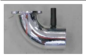
10. Cut the provided crankcase vent hose to a length of 1.75" and install onto the K&N® intake tube as shown.
