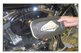
4. Remove the air filter as shown.
