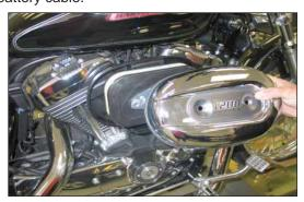
2. Remove the two air filter cover mounting bolts and then remove the cover from the vehicle as
