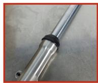
4. Install the RSD Fork Dust Cap by sliding it over the inner tube and pressing straight down. Be sure to apply even pressure all around, both 0 rings need to clear the groove. NOTE: Use very light lube if you are unable to seat both 0 rings.
