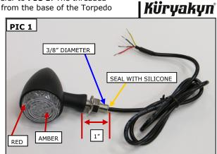
Use a test light and the wiring diagram for your bike to locate a ground wire; a "keyed" 12 volt power wire (a running light that has power when the key is "**ON**" and loses power when the key is "**OFF**"); the left and right turn-signal power wires; and brake light power wire. Record the color of the wires in the boxes below.
