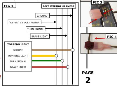
**TORPEDO LIGHTS with RUN-TURN-BRAKE FUNCTION**
