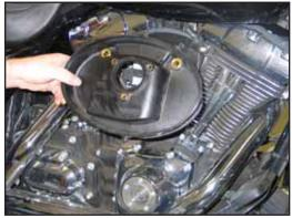
6. Remove the air filter base from the vehicle as shown.
