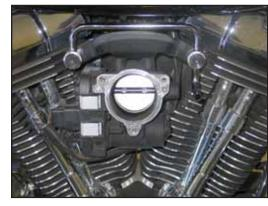
7. Install the supplied crank case breather tube using the provided breather bolts and washers.
