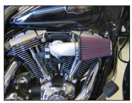
10. Install the provided K&N® air filter and secure with the provided hose clamp.
