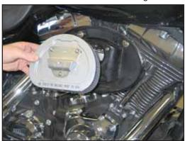
4. Remove the air filter from the vehicle and disconnect the crank case breather tubes.
