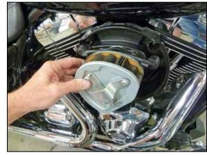
5. Remove the air filter from the vehicle and disconnect the crankcase breather tubes.
