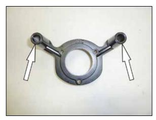
8. Install two of the o rings provided onto the back side of the  $K\&N^{\otimes}$  back plate as shown.
