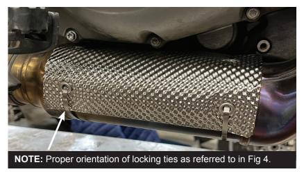
FIG 5 Route ties over and behind catalytic converter and start ties. Position shield properly as in this image and tighten ties.
