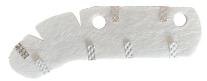
STEP 3. Fold the tabs of the aluminum around the Duraglass. Fig 2
