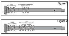
Prior to installing your Drop-In Fork Lowering kit, you **MUST REMOVE** any previously installed fork lowering kit components, such as the 1 or 2 additional top out springs illustrated above. Additional top out springs are common in many such kits.
