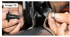
12. Install provided 45mm springs from muffler to slip-tube. (Reference image 10)
