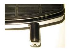
After drilling the holes, mount the body pieces of the footrest pegs to a desired position. Mount the sleeves and end pieces. Secure the screw joint by locking.
